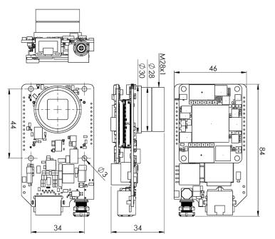
**T-REX EVO** is a highly customizable and user-programmable FPGA-based high-speed smart camera which features a high-end FPGA camera with a Xilinx Zynq FPGA and a high-speed imaging sensor and a Gigabit Ethernet. It includes ARM System-on-Chip (SoC) technology combined with a turbocharged industrial CMOS imaging sensor.
