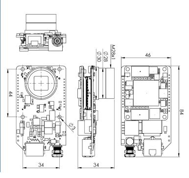
**Velociraptor EVO** is a highly customizable and user-programmable FPGA-based high-speed smart camera: the ultimate FPGA camera with a very large Xilinx Spartan-6 FPGA and high-speed imaging sensor. It is based on GigaBee modules which incorporate dual DD3 memory and Gigabit Ethernet. It features the ultimate-performance System-on-Chip (SoC) technology combined with the latest turbocharged industrial CMOS imaging sensor.
